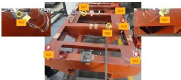
Fig. 10: Strain gauge locations on the chassis mounted platform
