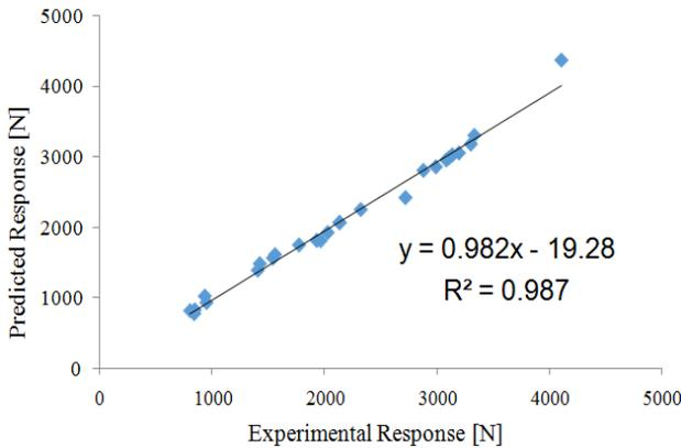
Fig. 3: Predicted vs. Experimental braking force values
