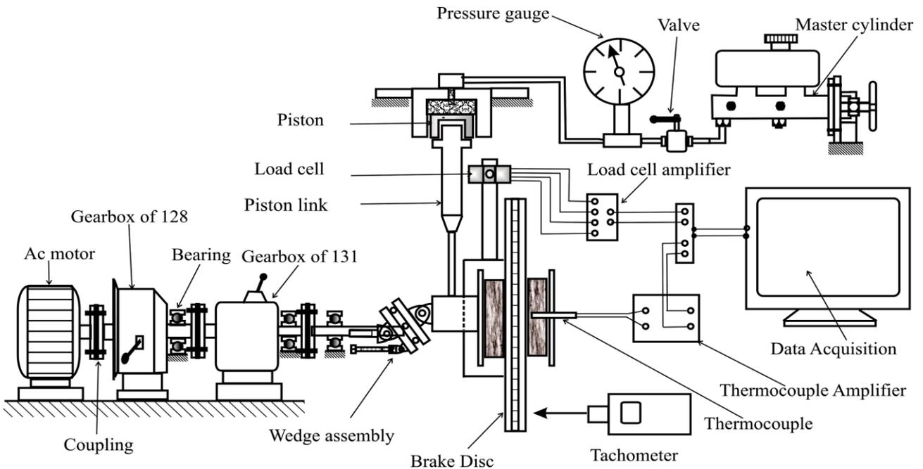
Fig. 1: Schematic of brake dynamometer test setup and measurement instrumentation
