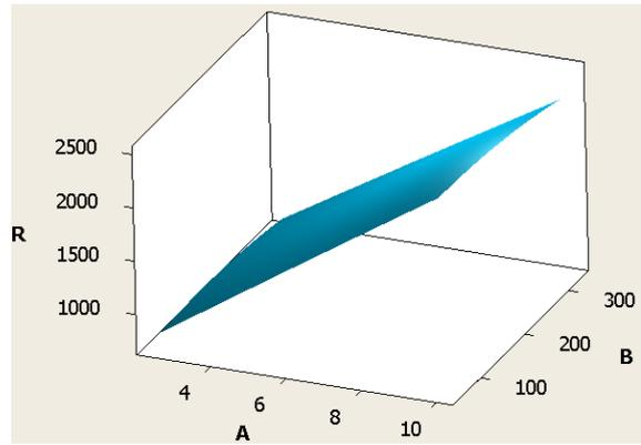
Fig. 4(a): Applied pressure and rotational speed vs. Braking force
