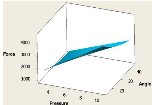
Fig. 4(b): Applied pressure and wedge angle vs. Braking force
