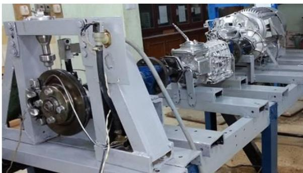
Fig. 2: Main components of the brake dynamometer
