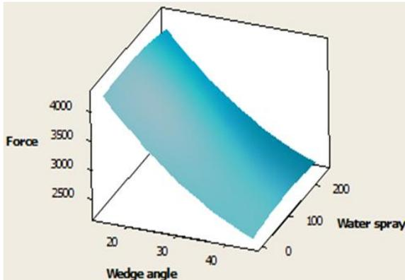
Fig. 4(f): Wedge angle and water spray vs. Braking force
