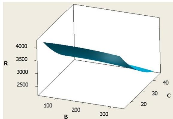
Fig. 4(d): Rotational speed and wedge angle vs. Braking force
