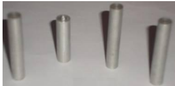
Fig. 1: Photograph of Al6061-SiCp MMC wear test specimens
