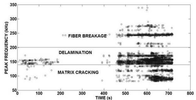
Fig. 5(a): Peak frequency vs. Time for pristine specimen
