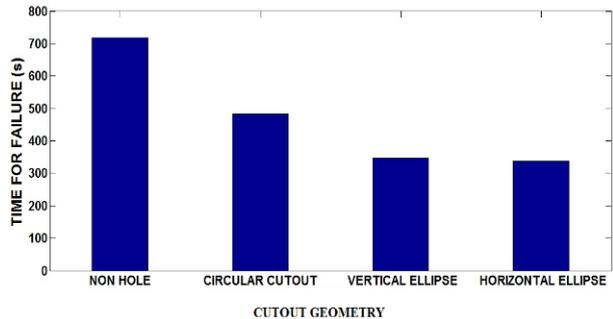
Fig. 8 (b): Time for failure plot for composite specimens
