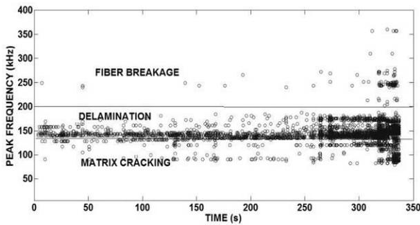
Fig. 5(d): Peak frequency vs. Time for horizontal elliptical cut-out specimen
