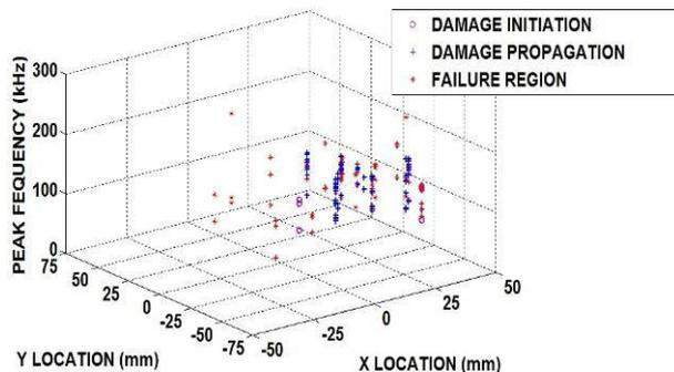
Fig. 9 (c): Peak frequency (kHz) vs. Location (X, Y) mm for vertical elliptical cut-out specimen
