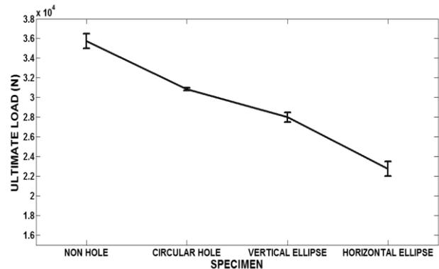
**Fig. 3:** Ultimate compression load form test of composite specimens
