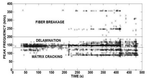
Fig. 5(b): Peak frequency vs. Time for circular hole specimen
