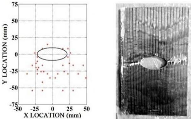
Fig. 4(c): Event location for horizontal elliptical specimen
