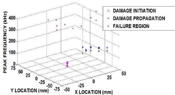
Fig. 9 (b): Peak frequency (kHz) vs. Location (X, Y) mm for circular cut-out specimen
