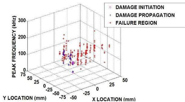
Fig. 9 (d): Peak frequency (kHz) vs. Location (X, Y) mm for horizontal elliptical cut-out specimen
