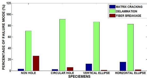
Fig. 6: Percentage of failure mode for composite specimens
