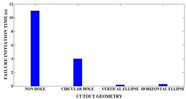
Fig. 8 (a): Time for damage initiation for composite specimens
