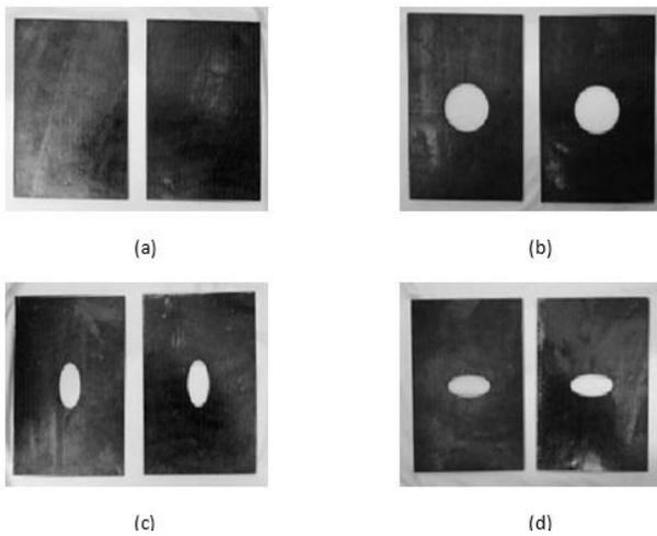
**Fig. 1:** Test specimens - (a) Pristine, (b) Circular hole, (c) Vertical elliptical hole, (d) Horizontal elliptical hole
