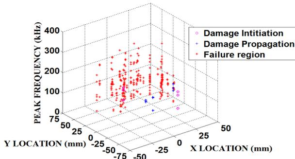
Fig. 9 (a): Peak frequency (kHz) vs. Location (X, Y) mm for pristine specimen
