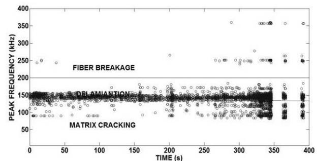
Fig. 5(c): Peak frequency vs. Time for vertical elliptical cut-out specimen
