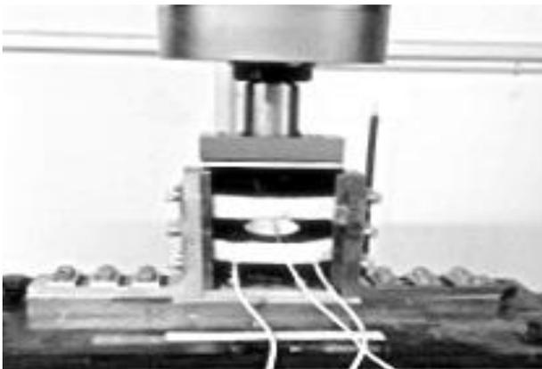
**Fig. 2:** Experimental setup of compression test
