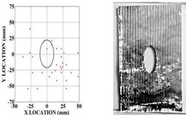
Fig. 4(d): Event location for vertical elliptical specimen
