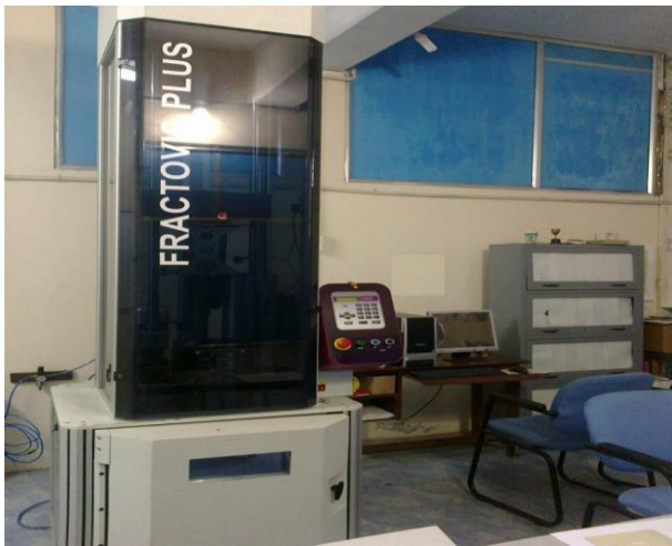
Fig. 1: Fractovis Plus drop weight impact setup
