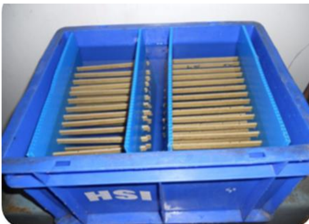
Fig. 2: GFRP specimens immersed in seawater bath
