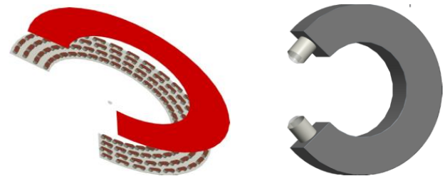
Fig. 4: Exploded views of customized TEG (left) & heat sink (right)
