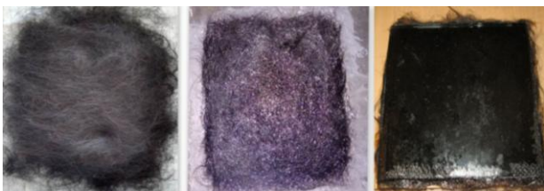
Fig. 1: (a) Goat hair layer; (b) Goat hair layer reinforced epoxy; (c) Compression moulded composite specimen
