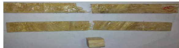
Fig. 5: Sisal fibre reinforced epoxy specimens after test
