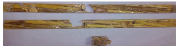
Fig. 7: Sugarcane fibre reinforced epoxy specimens after test
