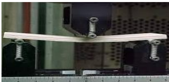
Fig. 4: Three point bending test setup
