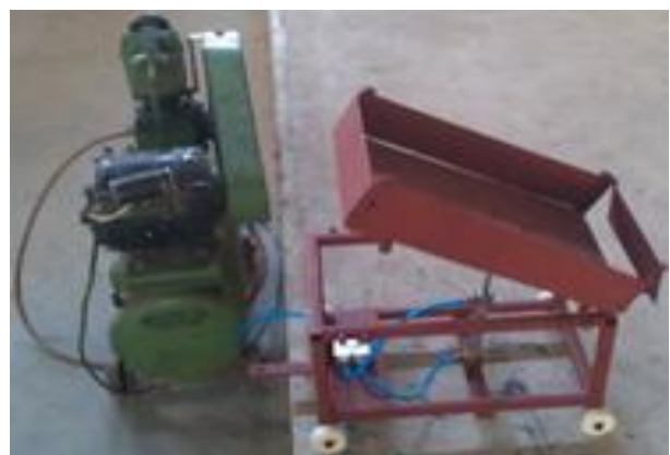
Fig. 5: Photograph showing dumper discharging front ways
