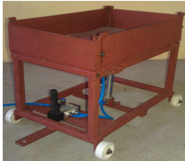
Fig. 4: Photographic views of the successfully fabricated innovative multi axis pneumatic dumper
