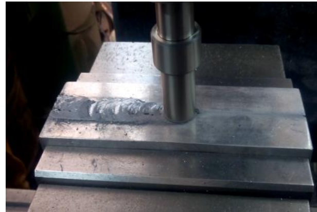
Fig. 3: FSP of hybrid composite during tool traverse
