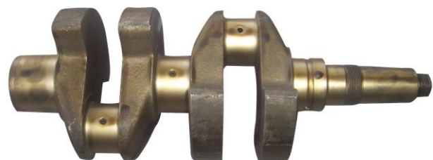
Fig. 1: Crankshaft example with 2 crankpins & 2 connecting rods
