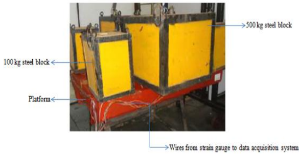
Fig. 7: Load distribution on the platform during experimentation
