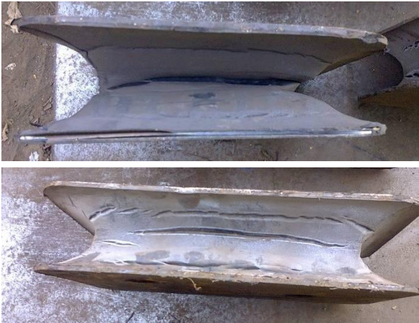
Fig. 3: Crack location on draft pad - Lateral orientation (top) and Longitudinal orientation (bottom)
