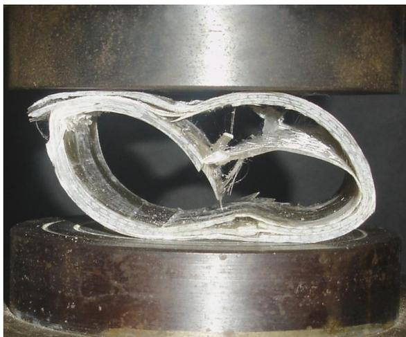
Fig. 5: Tested specimen - Lateral crushing
