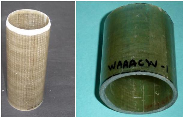
Fig. 1: Specimens for axial (left) and lateral (right) crushing
