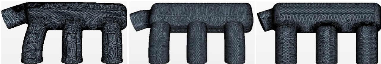
Fig. 2: Intake manifold runner grid models for scheme 1 (Left), 2 (Middle) & 3 (Right)
