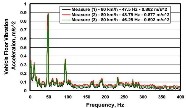
Fig. 4: FFT analysis of floor vibration acceleration in ORV interior at 80 km/h on coarse asphalt road
