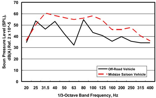
Fig. 11: 1/3-Octave band frequency SPL in ORV & MSV for vehicle speed 80 km/h on coarse asphalt road surface
