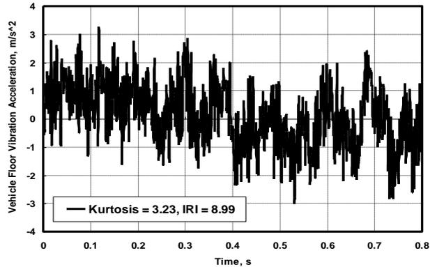
Fig. 12: Time history of the floor vibration acceleration in the MSV interior at 100 km/h on coarse asphalt road
