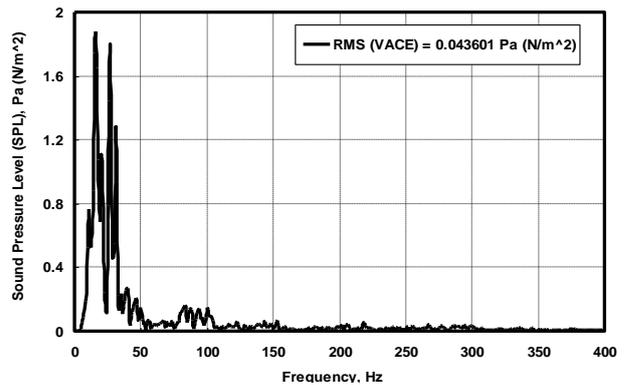
Fig. 13: FFT analysis of generated noise in MSV interior at 100 km/h on coarse asphalt road
