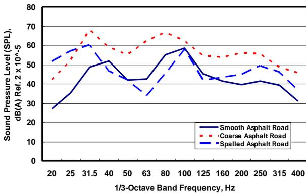
Fig. 9: 1/3-Octave band frequency SPL for MSV at vehicle speed 100 km/h on different road surfaces
