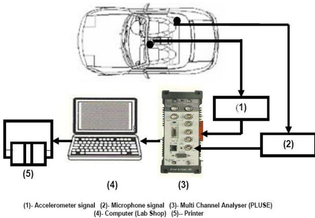
Fig. 3: Schematic of experimental setup
