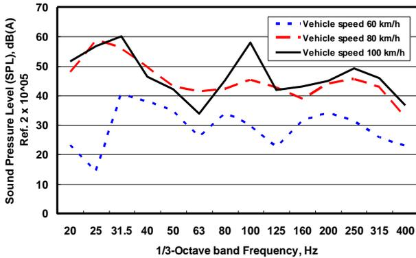
Fig. 8: 1/3-Octave band frequency SPL for ORV at different vehicle speeds on smooth asphalt road surface
