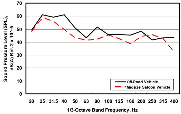
Fig. 10: 1/3-Octave band frequency SPL in ORV & MSV for vehicle speed 80 km/h on spalled asphalt road surface
