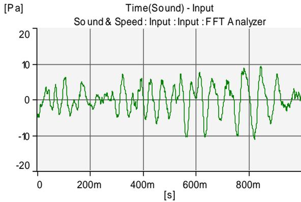
Fig. 7: Time history of MSV interior noise at 100 km/h on coarse asphalt road surface
