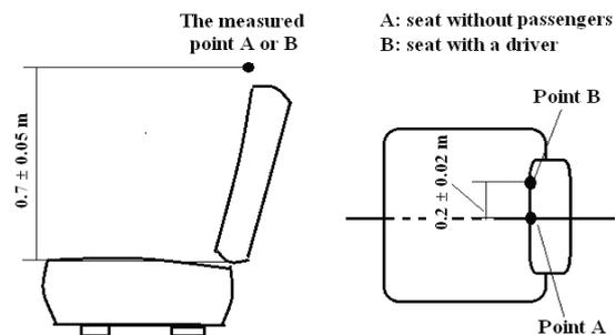
Fig. 1: Microphone arrangement for noise measurements
