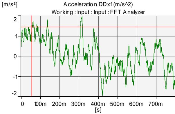
Fig. 6: Time history of MSV floor vibration at 100 km/h on coarse asphalt road surface
