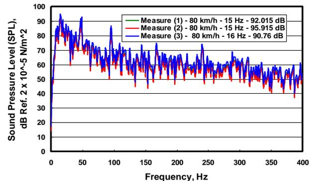
Fig. 5: FFT analysis of generated noise in ORV interior at 80 km/h on coarse asphalt road
