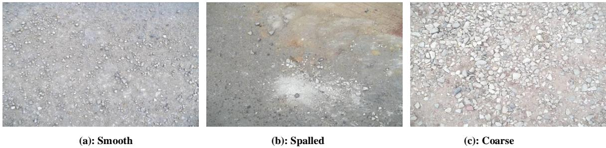
Fig. 2: Asphalt road surface roughness asphalt road surface
