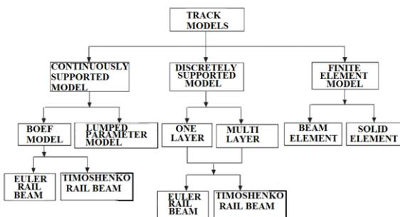
**Fig. 11: Model classifications for rail track**
