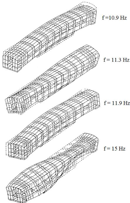
**Fig. 6: Four Eigen modes and corresponding Eigen frequencies for a free car body [10]**
