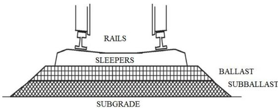
**Fig. 10: A typical track structure**
