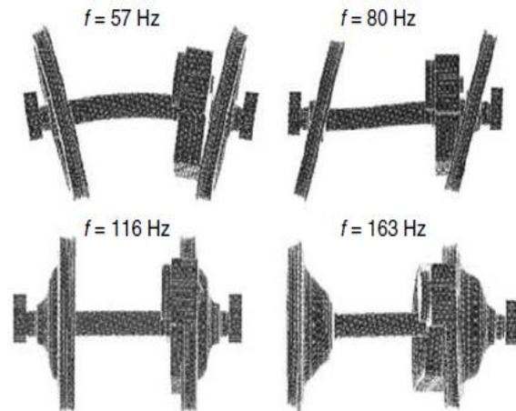
**Fig. 7: Four Eigen modes and Eigen frequencies for a free powered wheel set of diameter 1.3 m [47]**
