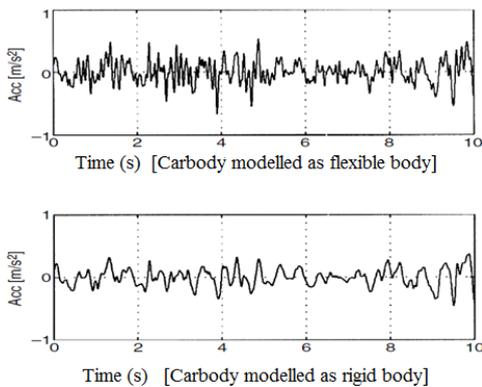
**Fig. 5: Simulated vertical acceleration on car body floor, middle position. Influence of structural flexibility [9]**
