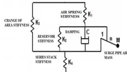
Fig. 4: Equivalent model of air spring arrangement
