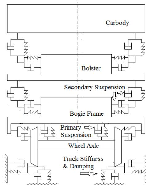
Fig. 1: Simplified view of a passenger rail vehicle [5, 6 and 10]
