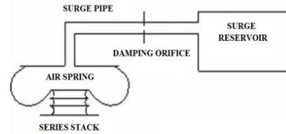
Fig. 3: Typical air spring arrangement
