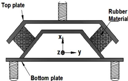
Fig 3: Engine mount system of the engine
