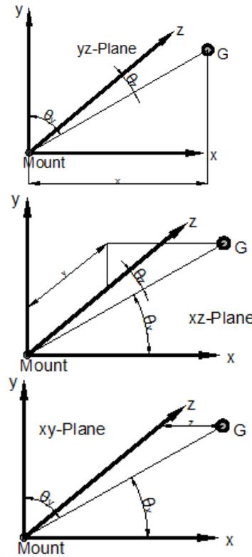
Fig. 4: Mount orientation with respect to engine mass centre
