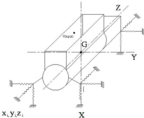
Fig. 1: Rigid body model of the engine-mount system
