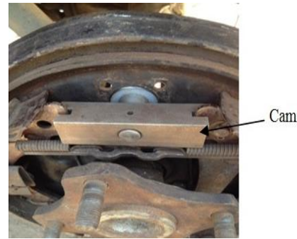
Fig. 1: Modification to drum brake system
