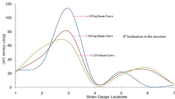
**Graph 1: Comparison of strain values for six degree (6°) inclination of the structure**
