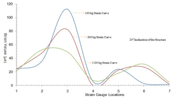
**Graph 3: Comparison of strain values for twenty degree (20°) inclination of the structure**
