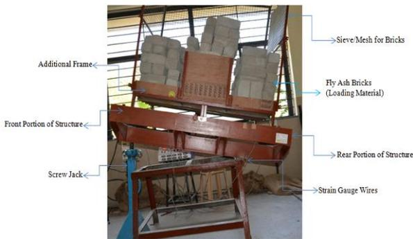
**Fig. 2: Experimental setup for gradient load strain measurement**
