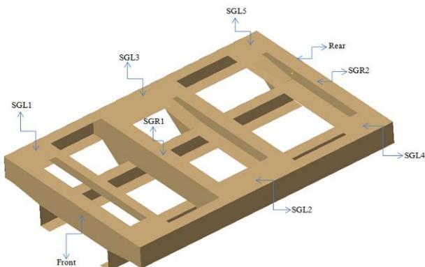
**Fig. 3: Positions of linear and rosette strain gauges on the structure**
