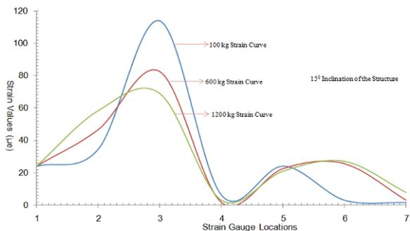
**Graph 2: Comparison of strain values for fifteen degree (15°) inclination of the structure**
