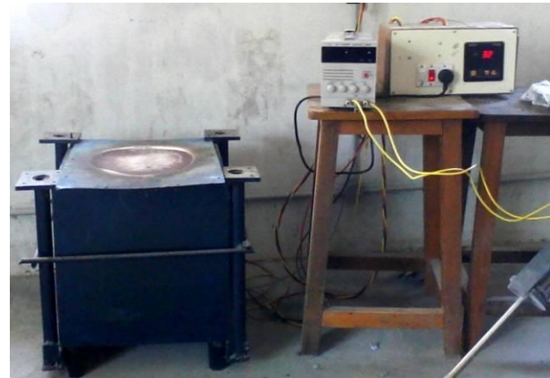
Fig. 1: Schematic of stir casting set-up
