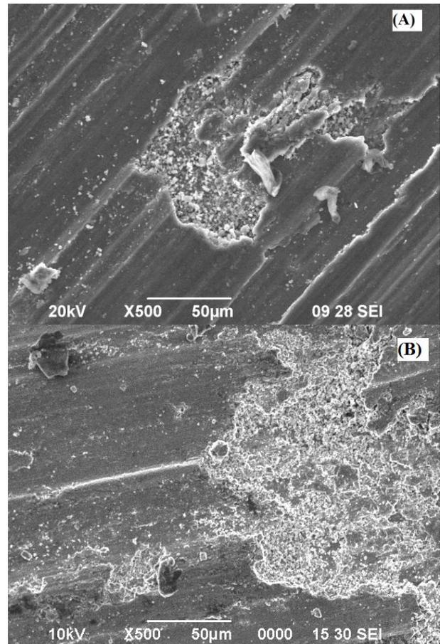
Fig. 7: SEM of the worn surface of AA6061 with 4% wt.  $ZrB_2$  and 5% wt. SiC AMC tested at normal load: (A) 10 N (B) 50 N
