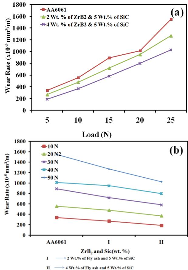
Fig. 3: Wear rate of fabricated AMC as a function of (a) ZrB<sub>2</sub> and SiC content and (b) Normal load
