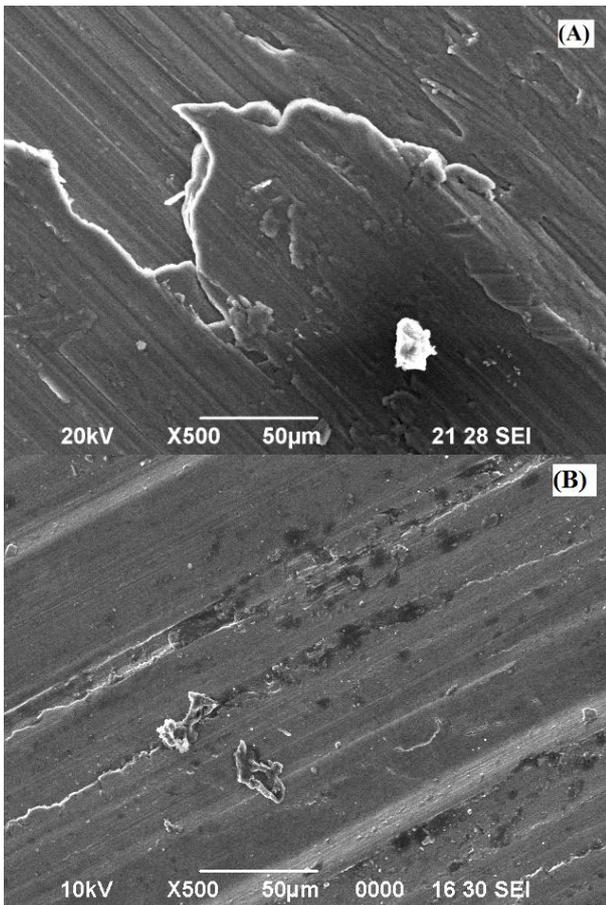
Fig. 4: SEM of the wear surface of the fabricated composite containing content of  $ZrB_2$  and SiC: (A) 0 % wt. (B) 4 % wt.  $ZrB_2$  and 5% wt. of SiC
