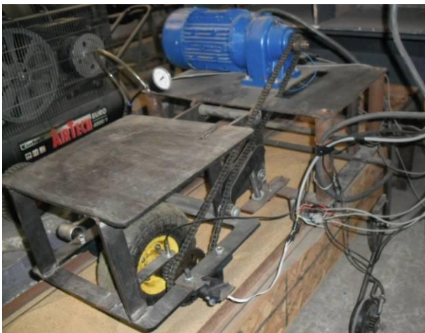
Fig. 1: Indoor soil bin facility test [14]
