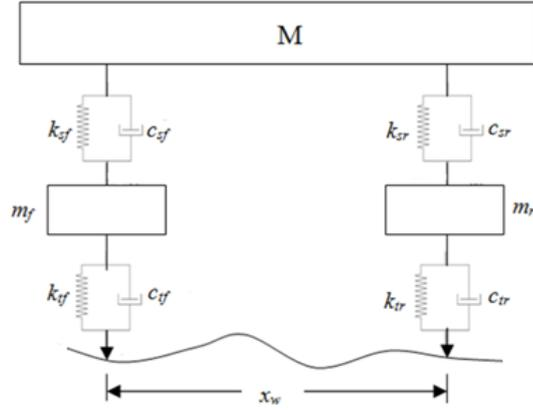
Fig. 6: Four wheel vehicle model (front view)
