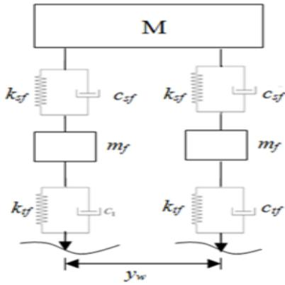
Fig. 5: Four wheel vehicle model (side view)
