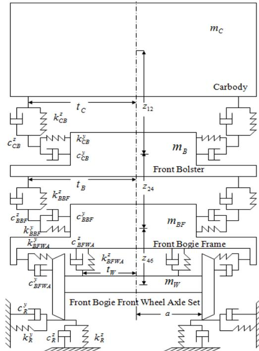
**Fig. 1: Rail-vehicle model (side view)**
