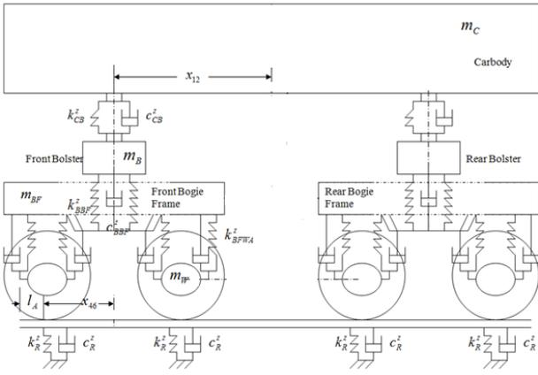
Fig. 2: Rail-vehicle model (front view)
