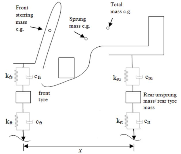
Fig. 4: Three wheel vehicle model
