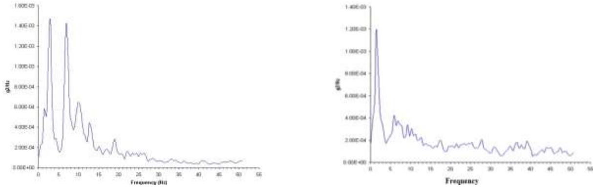
Fig. 4: PSD Curve for chassis mid portion left (CHM) on the platform, Paved road (Left) and Cross-country track (Right)
