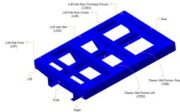
**Fig. 1: Accelerometer locations on chassis mounted structure for vibration measurement**
