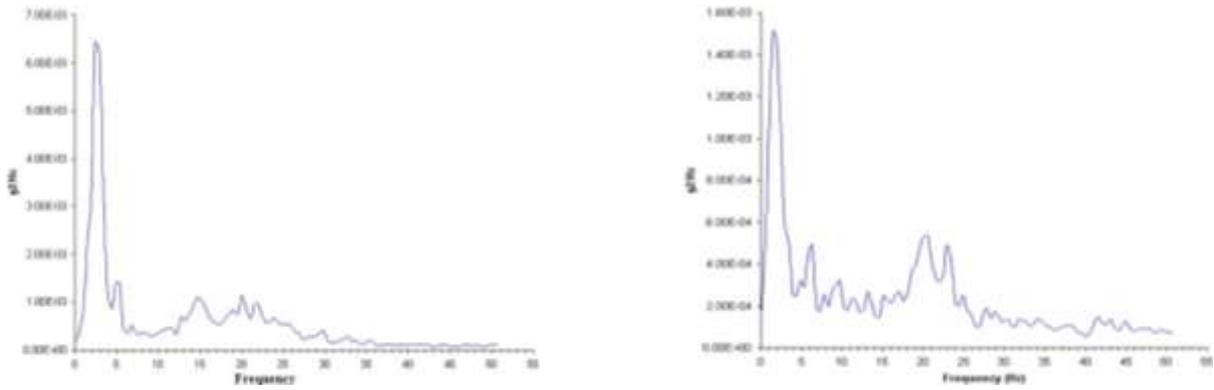
Fig. 3: PSD Curve for left side rear overhang portion (LSRO) on the platform, Paved road (Left) and Cross-country track (Right)
