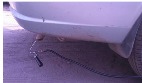
Fig. 6: The installation of probes in the vehicle
