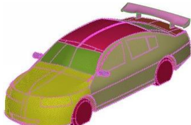
Fig. 5: Surface mesh of modified design
