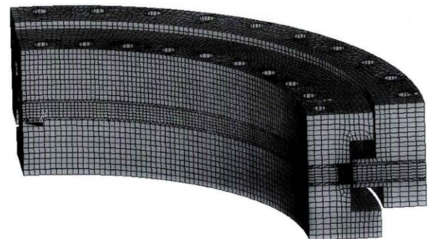
Fig. 4: FE model of three row cylindrical roller bearing
