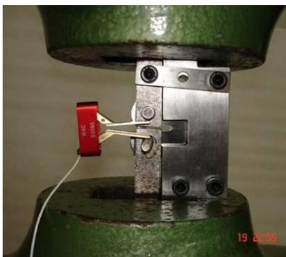
Fig. 2: Test set-up for fracture test
