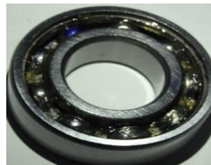
c). Ball defect (0.5 mm hole)
