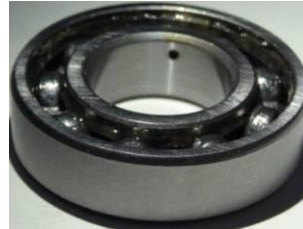
(b). Inner race defect (0.8 mm hole)
