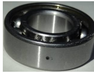
a). Outer race defect (0.8 mm hole)
