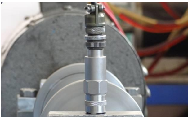
Fig. 4: Photographic view of accelerometer located on bearing
