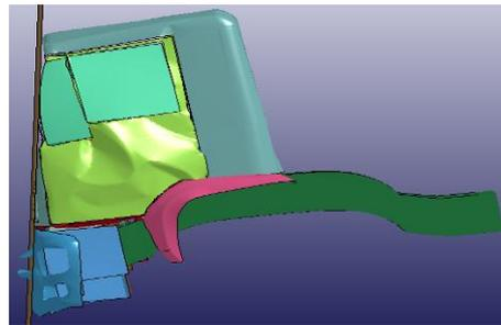
Fig. 10: Deformation of loaded cabin for Case-II at 100 milliseconds
