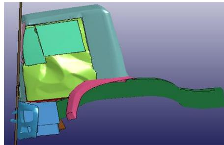
Fig. 11: Deformation of loaded cabin for Case-II at 200 milliseconds
