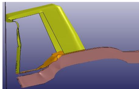
**Fig. 4: Deformation of bare cabin for Case-I at 200 milliseconds**
