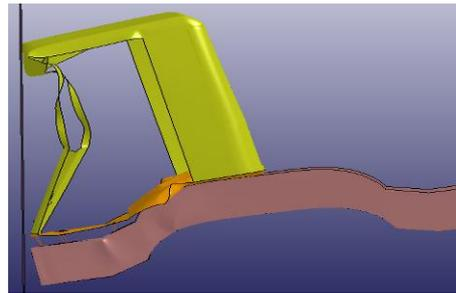
**Fig. 3: Deformation of bare cabin for Case-I at 100 milliseconds**
