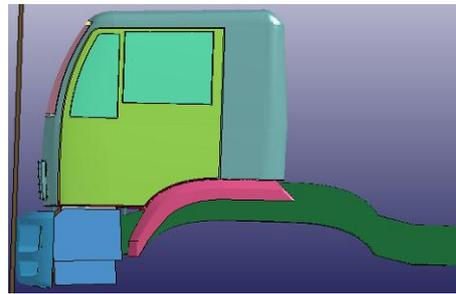
Fig. 9: Deformation of loaded cabin for Case-II at 0 milliseconds
