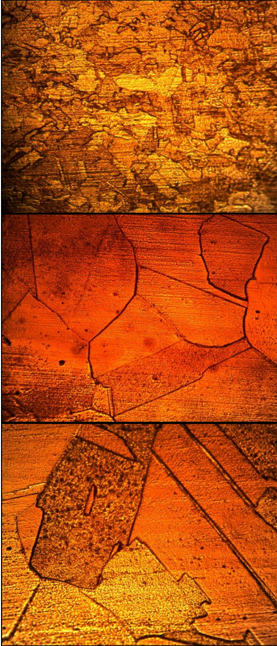
Fig 5: Optical micrographs of base metal (top) and different zones of CCGTAW (middle) and PCGTAW (bottom) joints
