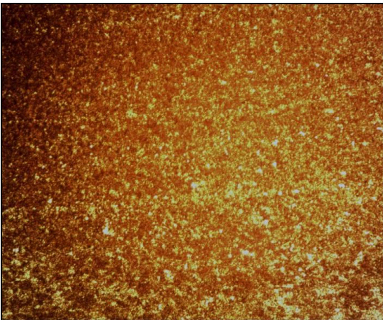
Fig. 6(d): Optical micrograph of FSW Joint - Stir zone
