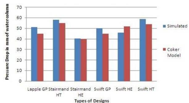
Fig. 3: Comparison between simulated and Coker models
