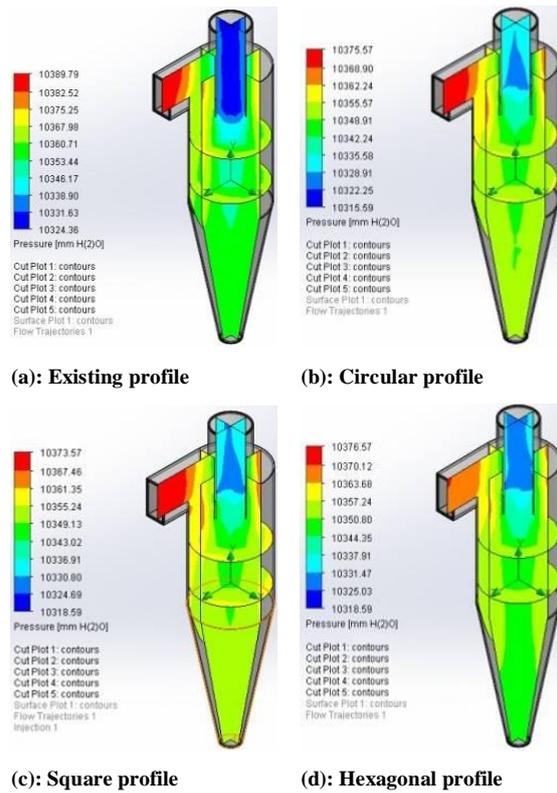
**Fig. 4: Lapple GP models – Pressure contours**
