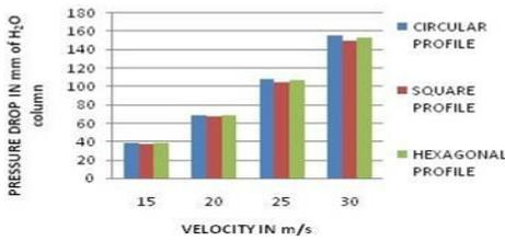
Fig. 5: Lapple GP pressure drop comparison
