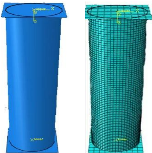
Fig. 1: Steel tube geometry and FE mesh of the model
