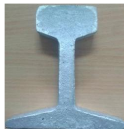
Fig. 4: Fabricated rail weld profile
