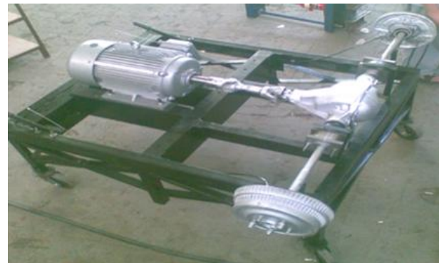
Fig. 3: Test rig of a rear axle of all wheel drive
