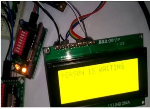
Fig. 4(a): Receiver - Request of the blind person in the bus module
