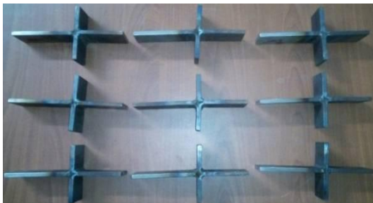
Fig. 6: Nine types of T-joint welds for testing
