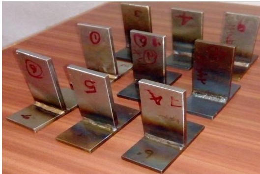
Fig. 5: Nine types of TIG welded T-joints
