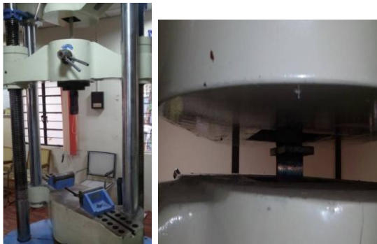
Fig. 7: UTM and specimen setup before test
