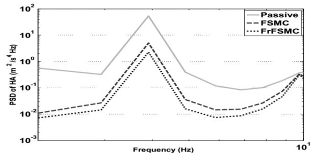
Fig. 17: PSD for sinusoidal road input
