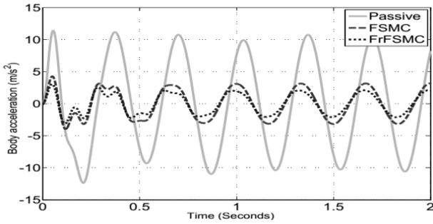
Fig. 10: Time response of the BA for sinusoidal road input
