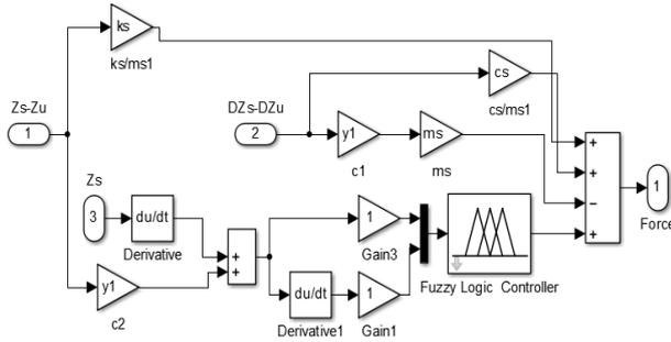
Fig. 5: Simulink model of the FSMC
