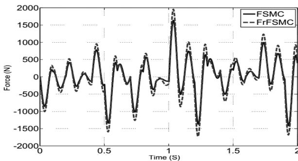
Fig. 13: Force produced by controllers for random road input
