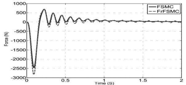
Fig. 9: Force produced by controllers for single bump input
