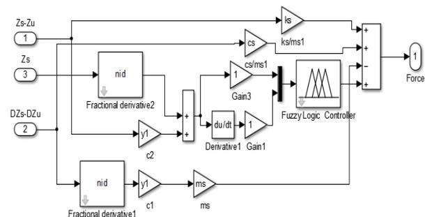
Fig. 6: Simulink model of the FrFSMC
