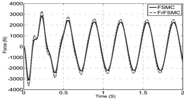
Fig. 11: Force produced by controllers for single bump input
