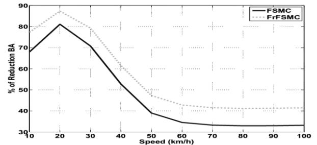
Fig. 15: Performance of the controllers with different speed of the vehicle for single bump
