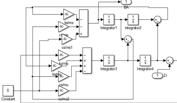
Fig. 4: Simulink model of the QCM
