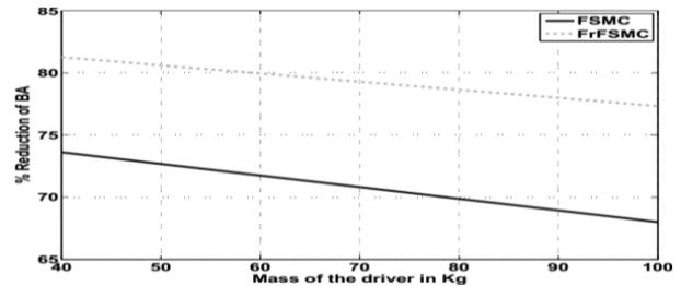
Fig. 14: Performance of the controllers with driver's mass variation for single bump
