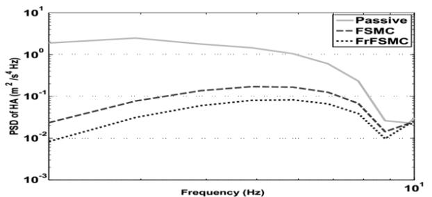
Fig. 16: PSD for single bump input
