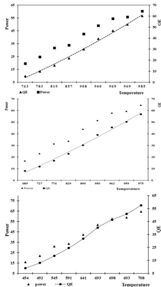
Fig. 2: Heat loss and power vs. Exhaust temperature outlet, Fuel types – Ron 95 (top), Ron 97 (middle) and Vpower (bottom)
