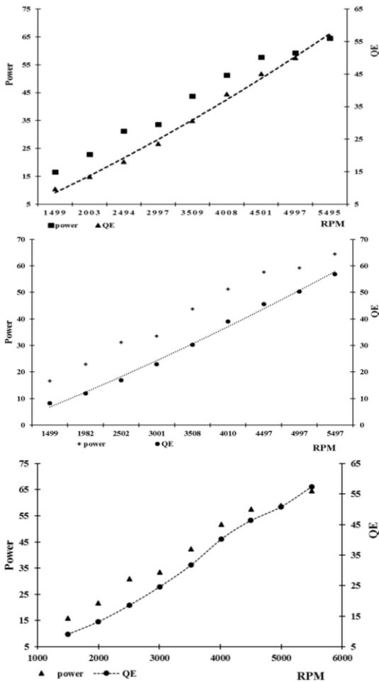
Fig. 3: Heat loss and power vs. Output in rpm, Fuel types – Ron 95 (top), Ron 97 (middle) and Vpower (bottom)
