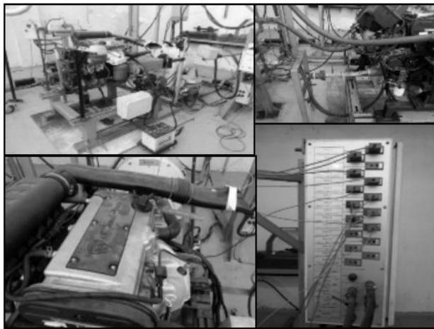
Fig. 1: Test setup of 1.6 CamPro Proton ICE and dynamometer
