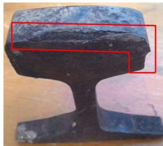
Fig. 1: Fatigue failure rail sample to identify initial damage development (UIC 54kg)
