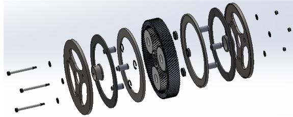
Fig. 8(a): Exploded view of planetary gear set
