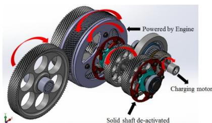
Fig. 3: Engine only with regeneration mode
