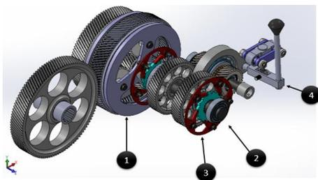
Fig. 1(b): Components of hybrid kit 1. Planetary gear set, 2. Shaft, 3. Ratchet and pawl, 4. Switching mechanism
