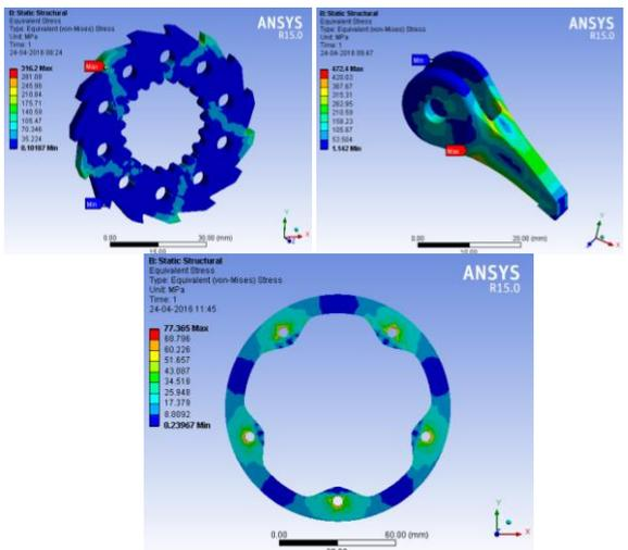
Fig. 12: Von-mises stress in sun shaft – Ratchet (top left), Pawl (top right) and carrier (bottom)
