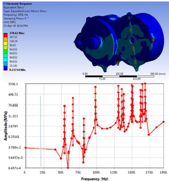
Fig. 15: Harmonic response analysis of Gearbox I & II
