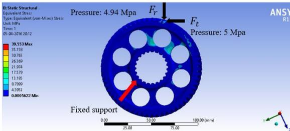
Fig. 11(b): Reduction gear analysis
