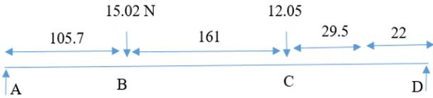
Fig. 7: Line diagram of sun shaft
