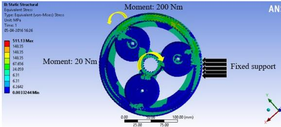
Fig. 11(a): Von-mises stress in parallel mode
