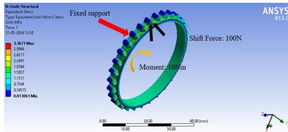
Fig. 13(b): Equivalent Von-mises stress in synchronizer
