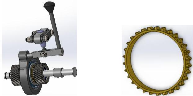
Fig. 9(b): Shifting assembly and synchronizer
