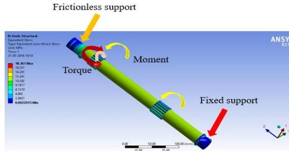
Fig. 14(a): Equivalent Von-mises stress in sun shaft when engaged
