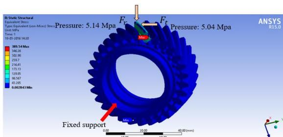
Fig. 13(a): Von-mises stress in shifter gear
