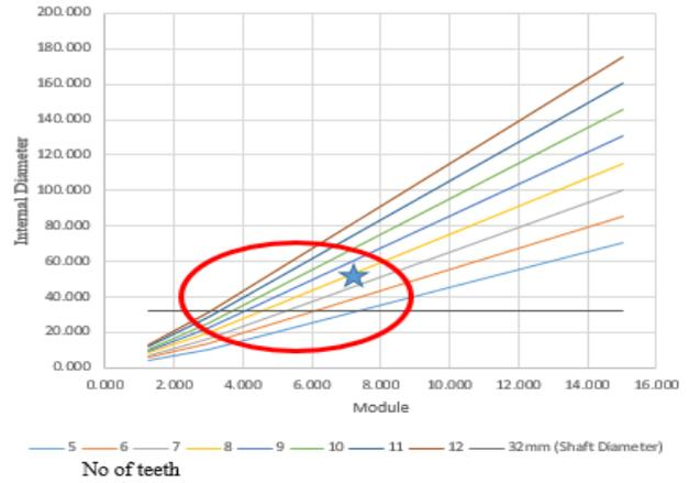
**Fig. 6: Graph for selection of ratchet’s module**
