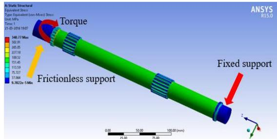
Fig. 14(b): Von-mises stress in sun shaft when dis-engaged
