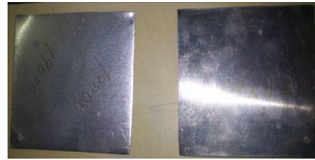
Fig. 6: Erichsen cupping specimen of dimension 90mm x 90mm
