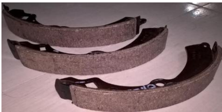
Fig. 1: Asbestos Brake lining Samples purchased for experiment
