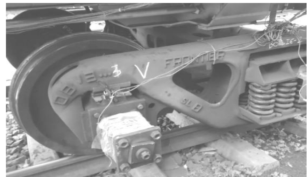
Fig. 18: Instrumented bogie frame for field trial
