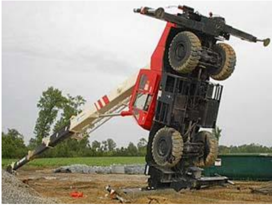
Fig. 2: Self-propelled vehicle tip over due do instability
