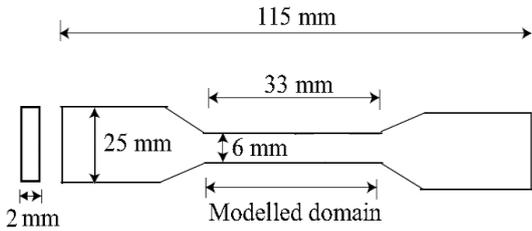
Fig. 2: Specimen dimension of NBR for tensile test
