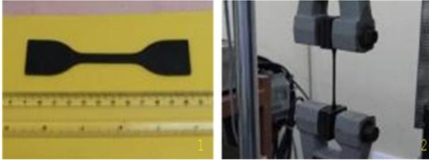
Fig. 3: Specimen of NBR for tensile test
