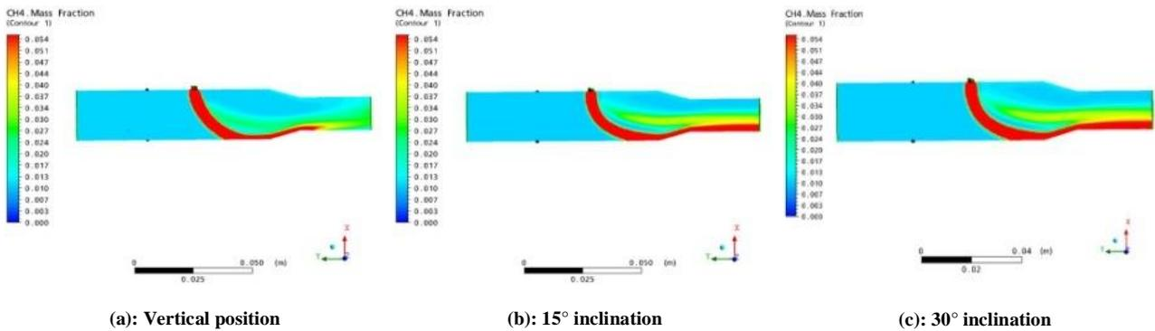
Fig. 3: Distribution of CH<sub>4</sub> mass fraction
