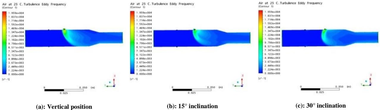
Fig. 5: Turbulence eddy frequency
