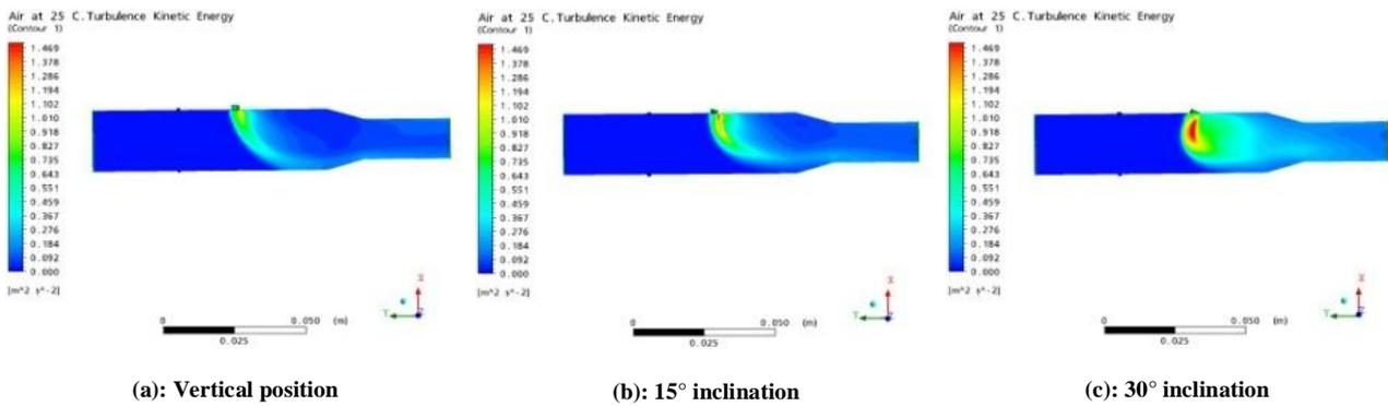
Fig. 6: Turbulent kinetic energy variation
