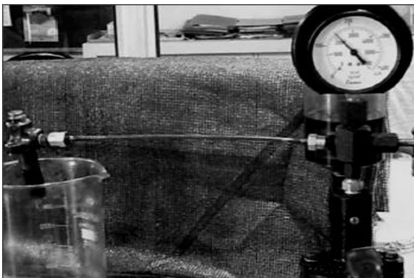
Fig. 3: Fuel injector while measuring IP
