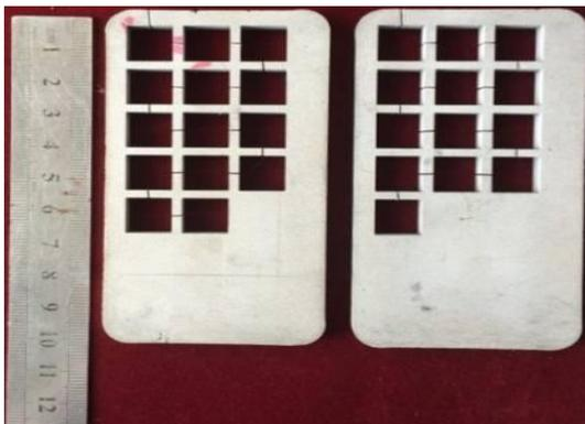
**Fig. 2: WEDM machined work pieces**
